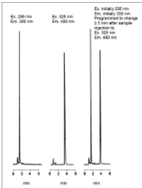
Figure 8. Chromatograms of serum extracts run on an HS-3 silica column using the Model LS-55.
