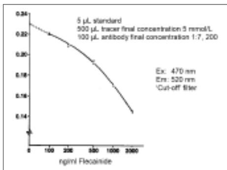
Figure 4. Polarization fluorescence immunoassay curve for the drug flecainide, using the Model LS-55.
