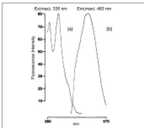
Figure 9. Fluorescence excitation a) and emission b) spectra of a quin-2/calcium complex.
