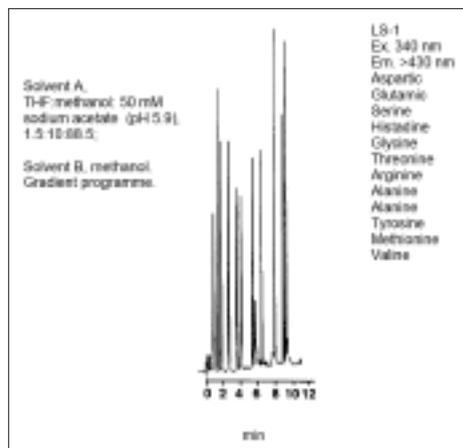
Figure 1. Chromatogram of amino acid standards derivatized by reaction with OPA, run on a 3 cm, 3 μ, C18 column.
