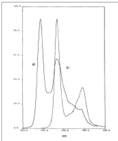
Figure 5. Fluorescence emission spectra of a) zinc protoporphyrin and b) protoporphyrin.
